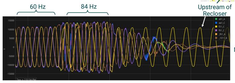
Recloser disconnected downstream sensors on all phases.
